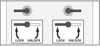
Figure 2. Configuration to lock the table so it is centered with the saw cabinet.
